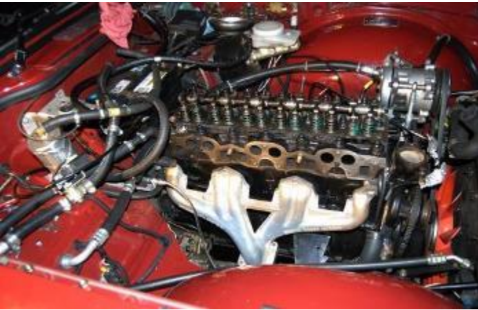
Above: Dean Tetterton's 1969 TR6 under repair due to a bent valve.
