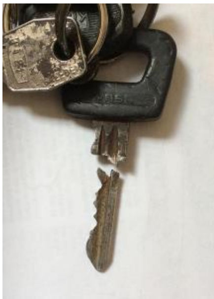
This is not Kenny's broken key, but it shows where later Spitfire, Stag, and TR6 ignition keys tend to break.
