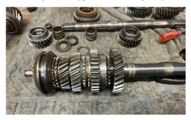
need to drop the laygear down in order to install the input shaft. The trick is to take an old laygear shaft and cut it off so it is just slightly shorter than the laygear, then install this shorter shaft into the laygear before dropping it into the case. The shaft
