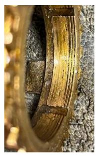
chro. Examination revealed I had mistakenly installed a worn synchro (from the pile of synchros on my workbench). As you can see in the photos, a good synchro will have distinct grooves on its interior face, while in a worn synchro these grooves are much less prominent.
