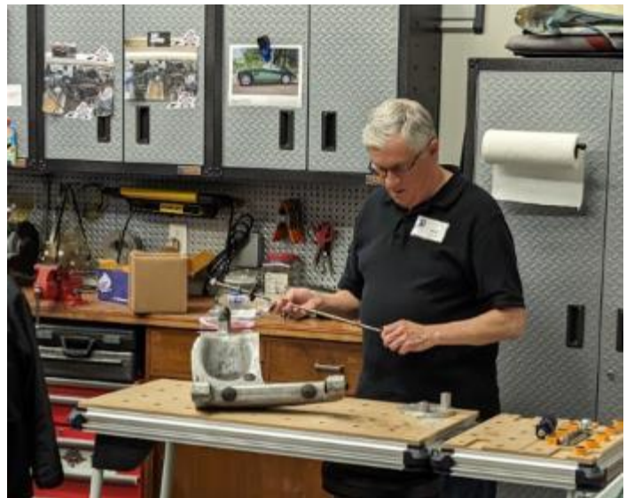
Don shows the threaded rod "hack" to removed old bushings from TR250s and TR6s.
